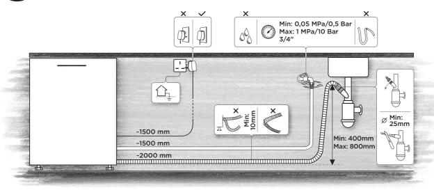
Refer to product specification sheet for cabinetry cut-outs. No connection behind the dishwasher supply 3/4 inch water tap.
