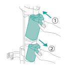
6 Place the empty dirty water tank back into the appliance and take out the clean water tank.
