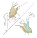
**3** Shake the foam filter over a waste bin to remove the layer of dirt on top of the foam filter. Then rinse the foam filter under a tap.
