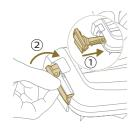
2 Slide the roller brush back into the LED nozzle (1) and push up the locking lever to lock the roller brush in the LED nozzle ('click').
