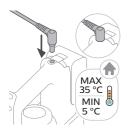
The appliance is equipped with a 25 V Li-Ion battery. Charging takes 4 hours.
