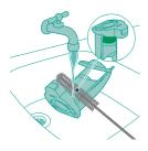
Clean the mesh part of the wet filter with the supplied cleaning brush.
