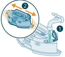
3 Fill the water tank with tap water and shake it over a sink.
