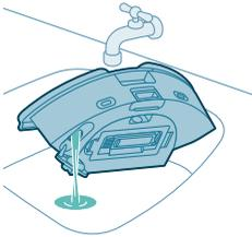
4 Pour out any remaining water in the water tank.
