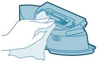
5 Dry the outside of the water tank with a cloth.
