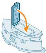
**12** Slide the dust bin back into the water tank.
