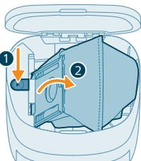
**2** Press the release button and push the bag holder to the side.
