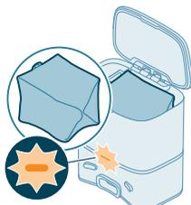
When the orange LED on the auto-empty station flashes indicating that the dust bag is full.
