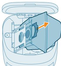
**3** Remove and dispose the dust bag.
