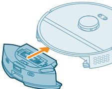
7 Insert the water tank in the robot.
