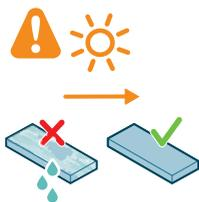
**8** Rinse the washable filter with water and air dry the washable filter.
