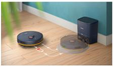
Experience uninterrupted cleaning with no battery worry, offering up to 130 minutes\* of runtime, enough for up to 120 m<sup>2</sup> on a single charge. When the battery runs low, the robot will automatically to recharge. Once the battery is charged, it will return to the place where it stopped to resume the cleaning.
