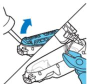
**9** Lift out the battery holder and cut the wires with a pair of cutting pliers or scissors.
