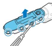
**8** Bend the snap hooks aside and remove the transparent cover of the power unit.
