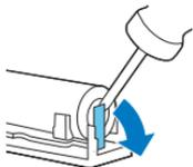
**10** Bend the battery tags aside with a pair of cutting pliers or a screwdriver.
