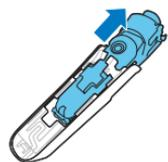
**7** Slide the power unit out of the body.
