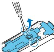
**6** Insert a flat head screwdriver on either side of the shaver body to release the hooks.
