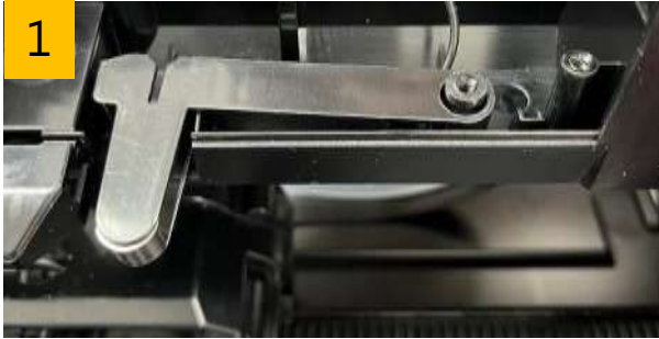
Install the charging contact, please pay attention to the wire color
