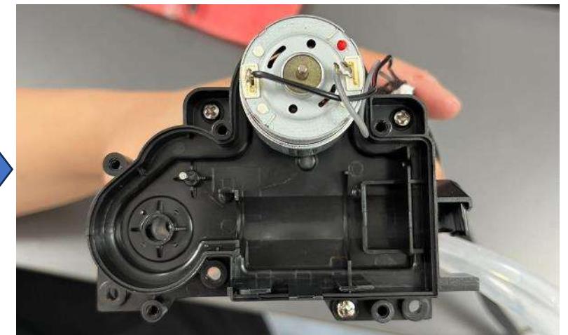
After removing the translation motor
