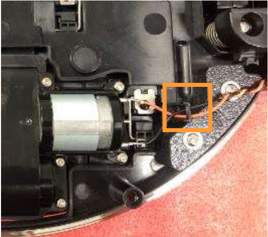
The wires should be organized and positioned at the original place
