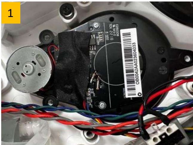
Put back the electrical tape and cover back. Fasten with 3 screws
