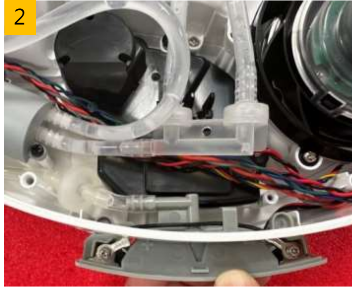
Remove inject water module and the pipes
