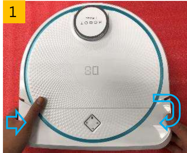
Remove the bumper by pressing one side
