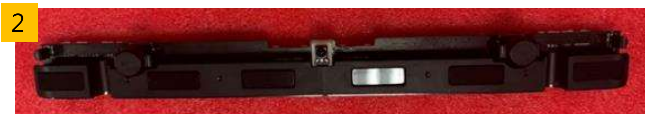
Remove the cover to fin the D8-Front PCB Assembly
