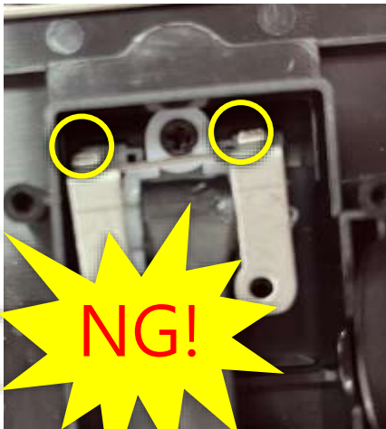
The metal hook should be tuck under the plastic
