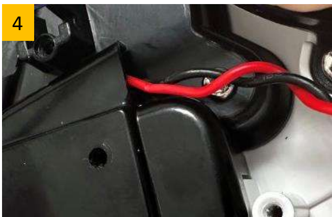
The wire need to pass through the cover.
