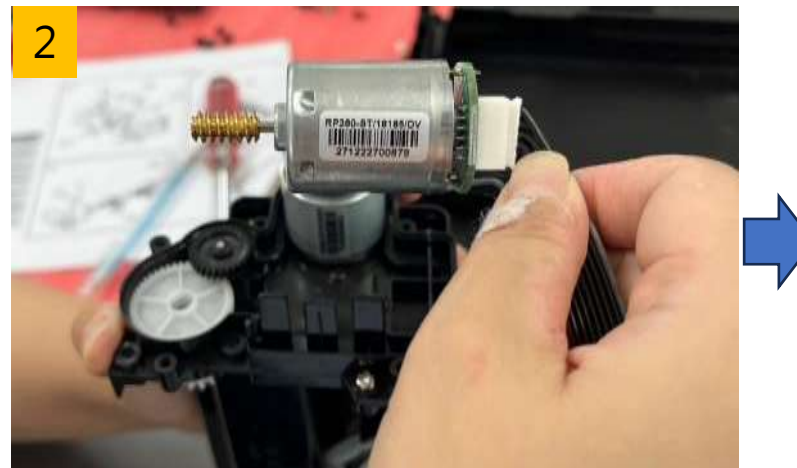
Disconnect the cable to remove the translation motor
