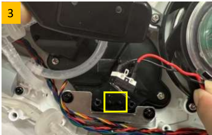
Install Lidar head hit sensor against to the pillars and cover back. Fasten with 3 screws.
