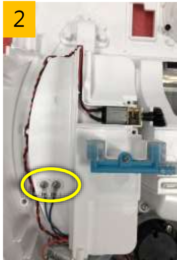
Remove 2 screws (the water level detectors) from the wires
