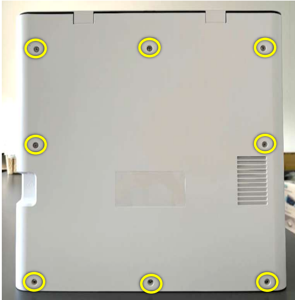
Unscrew 8pcs screws to remove rear cover
