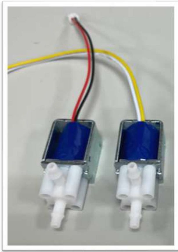
LuLu-Solenoid Valve_Refilling (Left side, red and blue wire)
