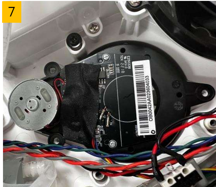
Remove the electrical tape
