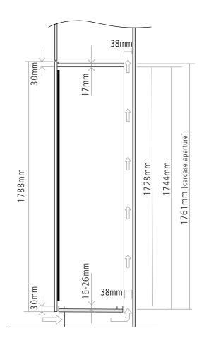
Please note: once installed the appliance door may not sit completely flush with the kitchen furniture door Dimensions may vary +/- 2mm due to manufacturing tolerances
