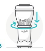
Place the lid back on the batchbowl and place the batchbowl assembly onto the motor base. Push down and twist clockwise to engage the motor. Blend until food reaches the desired consistency.
