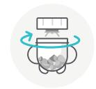
Twist the extractor blade onto the short cup ensuring it is sealed.
