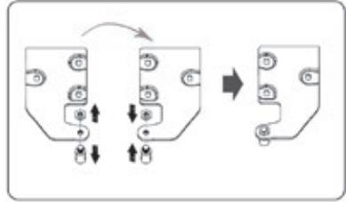
4. Loosen the screws supporting the middle door hinge and then remove the middle door hinge. Lift the refrigerator door about 50 mm to finally remove it from the unit.
