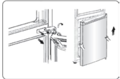
5. Remove the plastic cover on one side of the device and place it on the other side.
