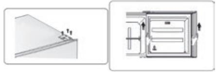
3. Loosen the screw on the door hinge and tighten it on the other side of the hinge.
