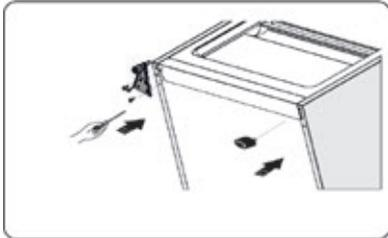
7. Unscrew the plastic plug and the screw on the bottom of the refrigerator door and replace them on the other side of the door.
