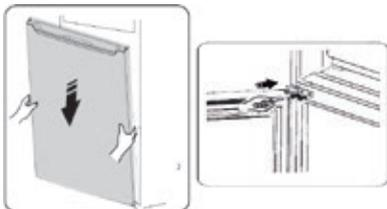
9. Loosen the plastic plug and the screw on the bottom of the freezer door and replace them on the other side of the door.
