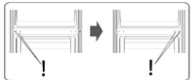
6. Tilt the device backwards slightly and remove the screws supporting the lower door hinge. Unscrew the adjustable stands and the possibly adjacent screws from the unit and screw them on the other side.
