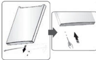
8. Attach the refrigerator door, rotate the middle door hinge 180 ° and then attach it on the opposite side of the unit. Attach the middle door hinge with the corresponding screws.
