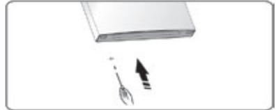
10. Replace the freezer door and mount the upper door hinge on the opposite side of the unit. Secure the upper door hinge with the corresponding screws.
