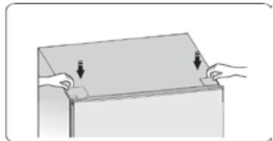
12. Finally, check the correct alignment of the doors. Make sure they are tightly sealed on all sides. If necessary, align the front feet of the appliance, so they are in a horizontal position.
